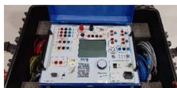
Three Phase Secondary Injector ISA
